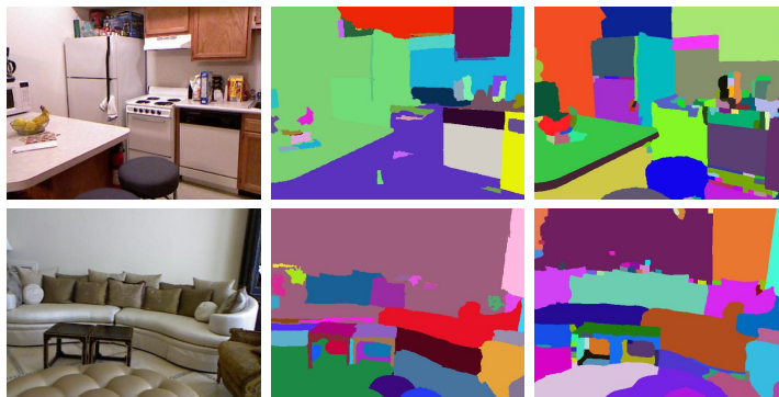
Fig. 2: Two examples to illustrate the benefits of using depth information. The first column contains two original RGB images from Kinect. The second column is the segmentations only based on RGB information. The third column contains the corresponding segmentations based on both RGB and depth information.
